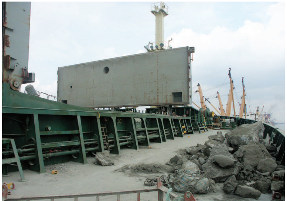
▲ Figure 2 Lumps of concrete within cement in bulk which is otherwise free running in a hold will cause difficulty and possible harm during discharge, in addition to reducing the value of the consignment.
