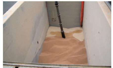
▲ Figure 2 Lumps of concrete within cement in bulk which is otherwise free running in a hold will cause difficulty and possible harm during discharge, in addition to reducing the value of the consignment.
