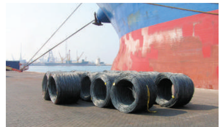
▲ Figure 4 The condition of wire rod in coil may change very slightly during carriage by ship, but it should not be wetted by sea water.
